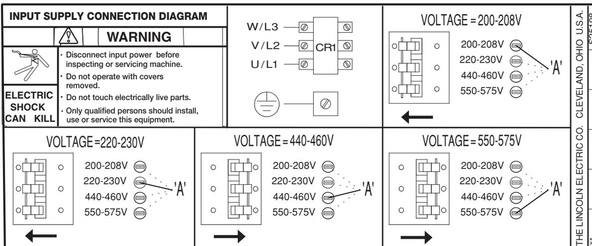
**NOTE:** Turn main input power to the machine OFF before performing connection procedure. Failure to do so will result in damage to the machine.
