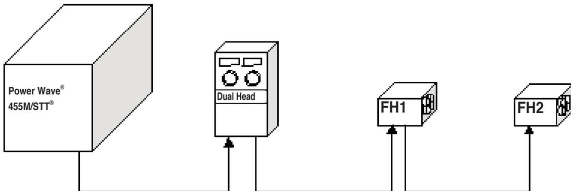
In this case the individual feed heads need to be assigned to the dual head control and the PW455 auto mapping disabled and the Equipment Groups set on (See figure A-6). (See the Feeder documentation for information on setting the feeder DIP switches)
