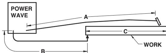
For long work piece lengths, a sliding work connection should be considered to keep the total welding loop length less than 50 feet. (See Figure A.3.)
