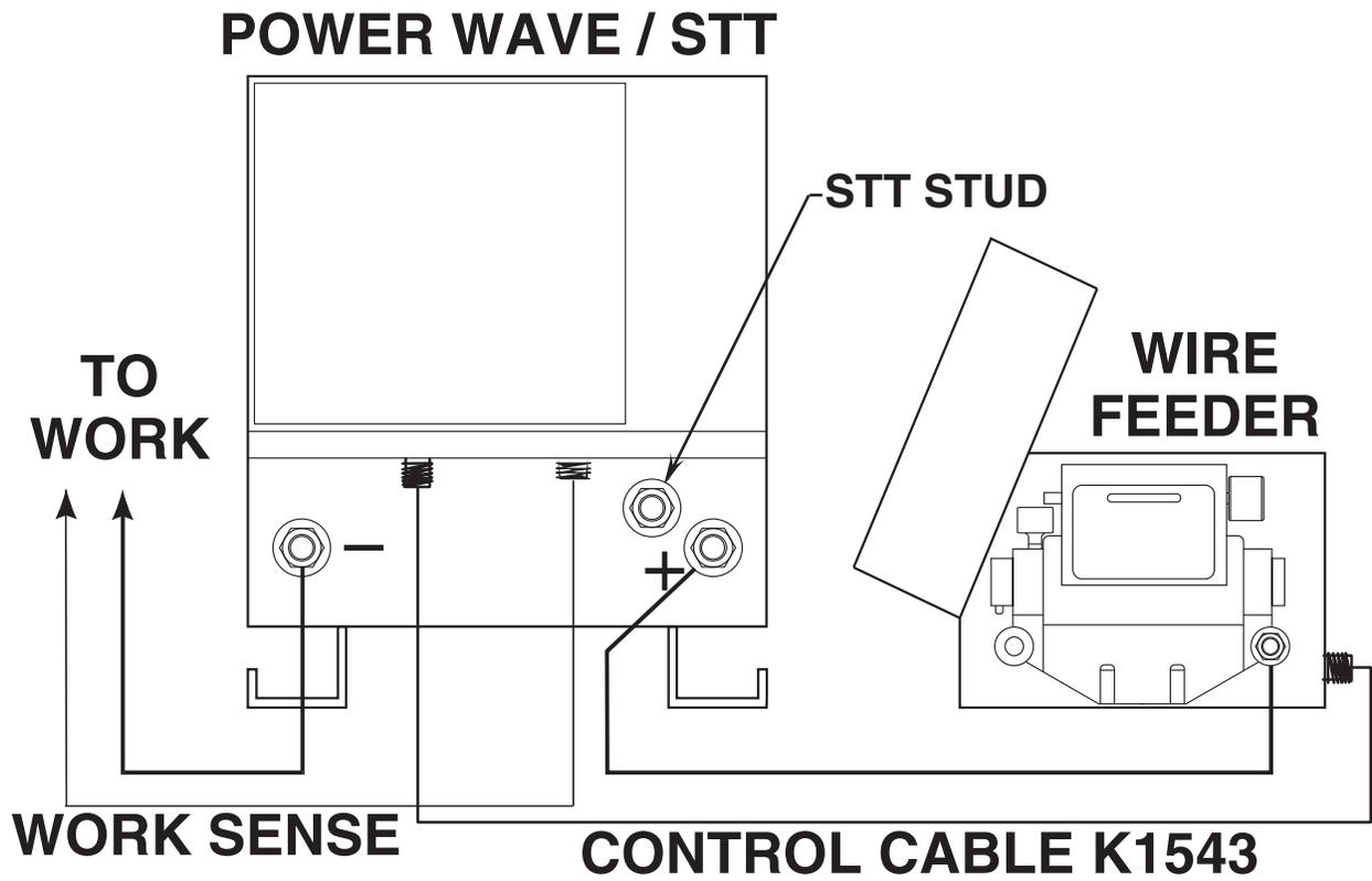
Connection Diagram Semi-automatic "Simple System"
