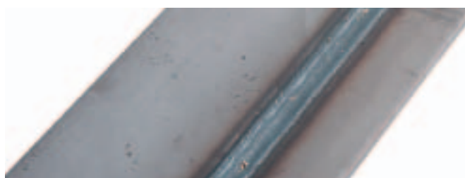
3/16" (4.8 mm) Horizontal Lap Weld
