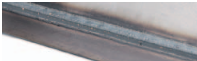
This thin gauge lap weld was made at a travel speed of 100 ipm
