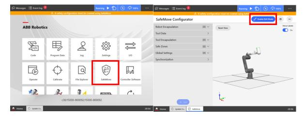
Select the three dots in the top right corner and from the dropdown list choose 'Load Configuration From File'
