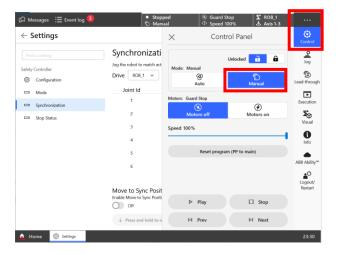
Toggle Enable Move to Sync Position to On.
