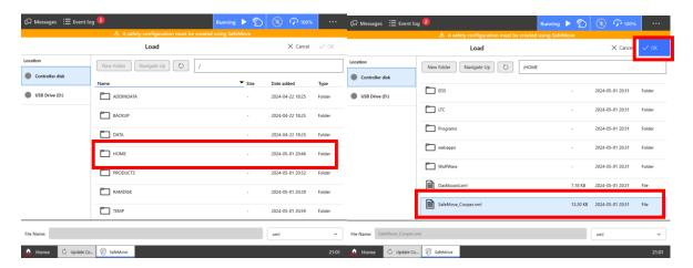
Select Write to Controller. The following screen will list all information related to the safety configuration. Select Apply to Controller. After being applied, you will be prompted to restart the controller. Select Restart Controller.
