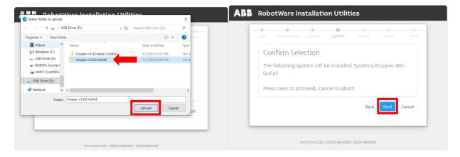
Note: If RobotWare Installation Utilities presents the message, "The controller contains no RobotWare System or current system is corrupted. Please install a new system before processing." Reattempt Section 3.1. If unsuccessful more than five times, contact support.
