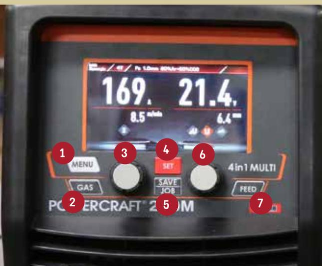
1. Welding mode button (press to select): Stick DC / TIG HF / TIG Lift / MIG Manual / MIG Synergic welding mode.
