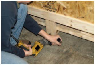
4. Carefully slide the crate assembly from the VRTEX™ 360.
