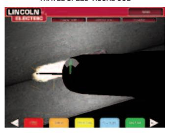
The CTWD (Contact To Work Distance) cue is only available for processes using the VR GMAW and VR FCAW gun. This cue uses color and position to indicate proper CTWD. The goal is to get the tip of the green arrow on the line of the "H" bar and keep the arrow color green.
