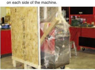
6. Carefully remove the post (long rectangular shaped cardboard box) from the crate.
