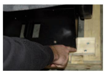
11. Remove the wooden cross brace while ensuring the unit is steady and secure.
