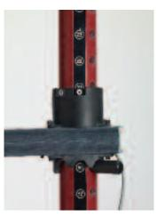
Note: If the table height indicator in the software cannot be moved to the pin height indicated on the post, move the arm height indicator in the software to a higher position and try again. See Troubleshooting Guide if necessary.
