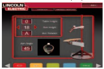
The physical stand should match the stand image when these selections are completed. To continue, press the green continue button. The stand setup verification screen will be displayed. This screen serves as a reminder to make sure VR stand components match the screen. When verified, press the green continue button again.
