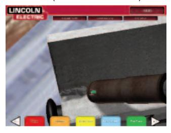
The **Arc Length** cue is similar to the CTWD cue but represents arc length distance for the VR SMAW process. The goal is to get the tip of the arrow on the line and keep the arrow color Green.
