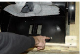
10. Remove the four screws from the wooden rear cross brace.
