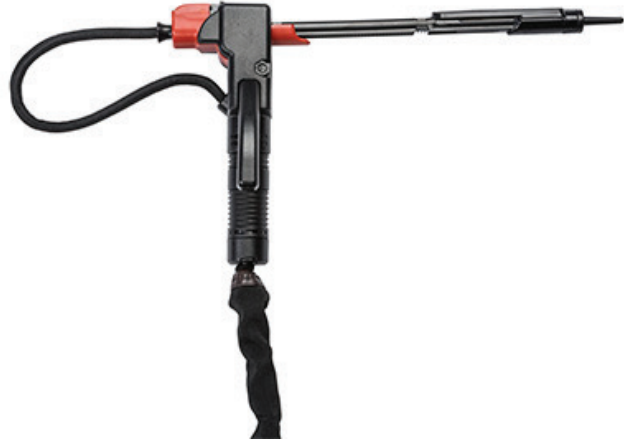
Figure 8 – VR SMAW device
