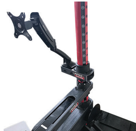
Figure 24 – Top pole section installation
