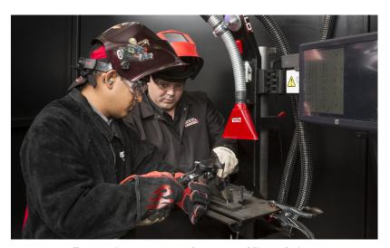
REALWELD allows an instructor to teach correct welding techniques and then have the student practice in Arc ON or Arc OFF mode with performance monitoring.
