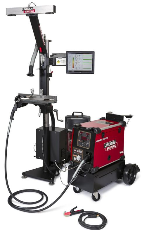
The REALWELD system is available as a standalone system to use with existing welding equipment or as a complete package with a Lincoln Electric Power Wave® C300 multi-process wire feeder/welder with necessary accessories.
