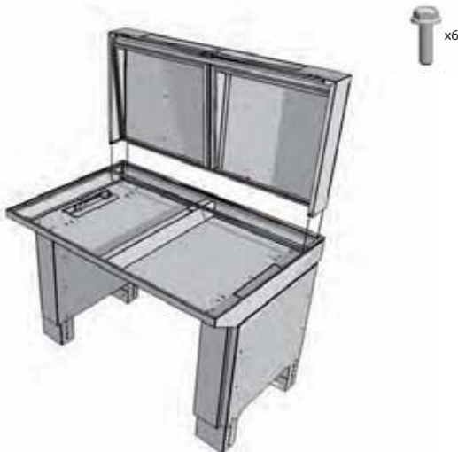
Figure A.4 - BACKDRAFT PANEL
