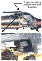
Screw adjusted out of trigger.
