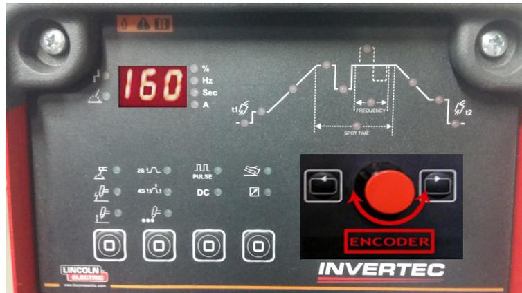
**4. STEP:** Setting min. current: Adjust with „ENCODER„ on value 4,3 AMP (+0.5 -0) on the clamp A-meter. If you have right value then push and hold „T6“ button till will be beep. Display shows „CAL„ and after „- - -“. For finish push „T1“ button. Min. current is set.
