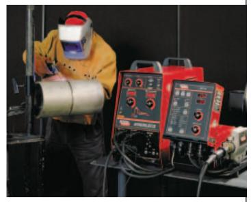
After each root bead, the capping pass is welded with the same parameters as the root pass by weaving the torch to fill up the joint. This operation has been automated to start the weaving automatically upon completion of the root pass. With STT<sup>®</sup>, penetration is outstanding with an excellent back bead, and a smooth, polished finish on the cap pass is obtained.
