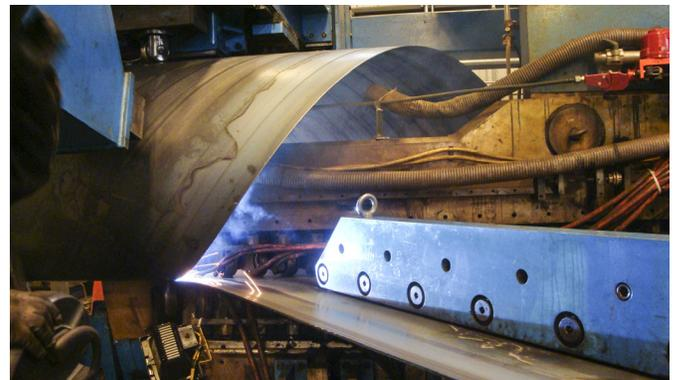
Welding speeds have nearly doubled at the tacking station via a unique setup using the Power Wave® AC/DC 1000® SD power source from Lincoln Electric.
