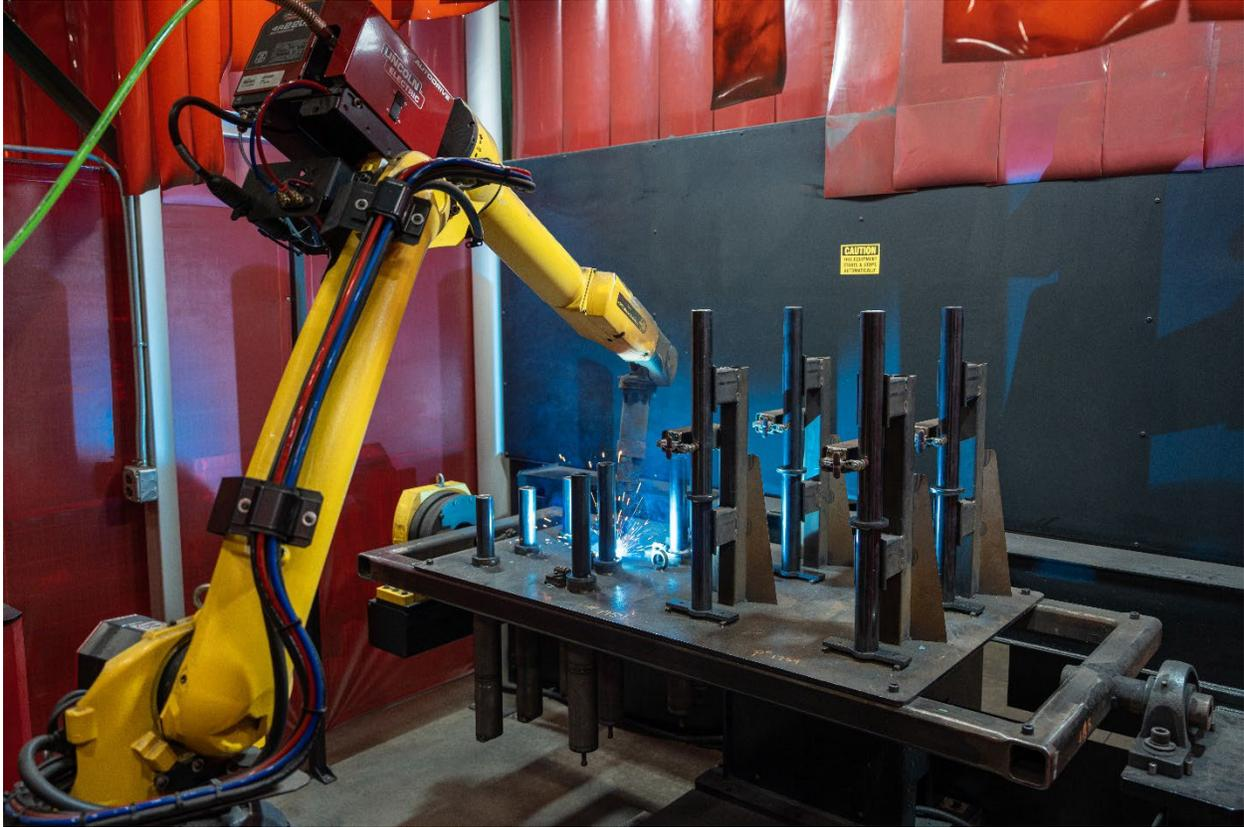
*Fab-Pak FHS-SS robotic welding system welds parts at Hickey Metal Fabrication*
