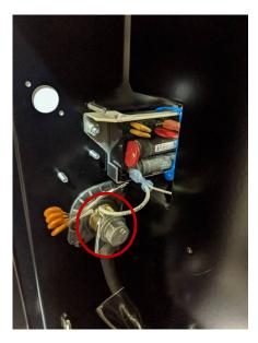
• Add a nut (9SCF000010) to the PEM stud, then attach the snubber cap, then add a lock washer (9SE106A-1) and a second nut (9SCF000010).
