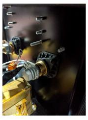
• Add a nut (9SCF000010) to the PEM stud, then attach the snubber caps, then add a lock washer (9SE106A-1) and a second nut (9SCF000010).
