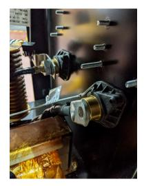
• Add one snubber cap assembly (9SS18858-26) to the output stud, between the lock washer and snubber lead terminal.
