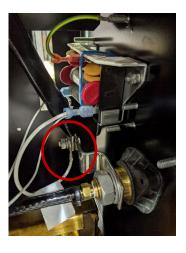
• Add 9SS18858-26 snubber cap assembly to bus bar.
