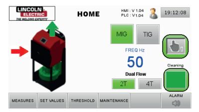
These maintenance alarms indicate that the run time counter of the relevant part has reached the limit and maintenance is required; the counter must then be reset up to the next cycle.
