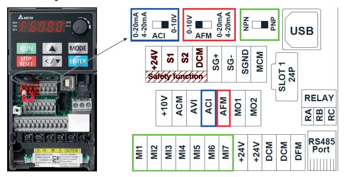
The switches for setting up the variator inputs and outputs must be set as follows:
