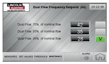
(1): the nominal extraction speed and the second speed dedicated to the Dual Flow mode are preset in the factory. These can however be changed from the Settings and Variator pages of the system configuration menu.
