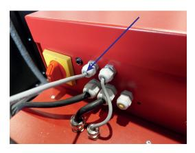
The automatic starting up of the **Linc Extractor** can be put under the control of any robotic, automated or other machines, by adding an external dry contact (contact closed = ON/contact open = OFF).
