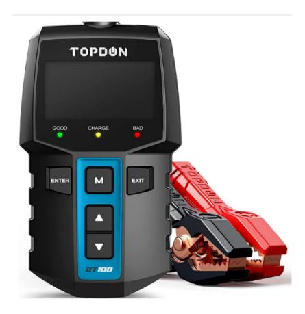
Use a load tester similar to the above testers to determine if battery is good.
