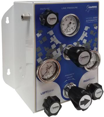
The SG 920 BR / SG 920 SS semi-automatic high purity switchover prevents downtime by automatically switching gas supply from the primary cylinder bank to the reserve cylinder bank. The user resets the primary bank by turning the knob. Manual adjustment of the individual regulators is not required. **All systems include a line control regulator.**
