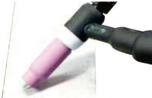
(13) Lay the outside edge of the cup on work piece with the tungsten Electrode 1~2mm from the work piece. Press and hold the trigger button on TIG torch to start the gas flow.
