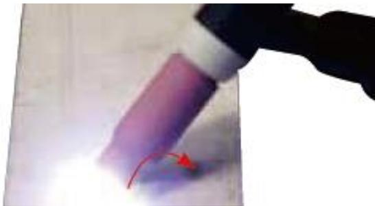
(15) Now rotate the Gas Cup in the reverse direction to lift the Tungsten electrode from the work piece to create the arc.
