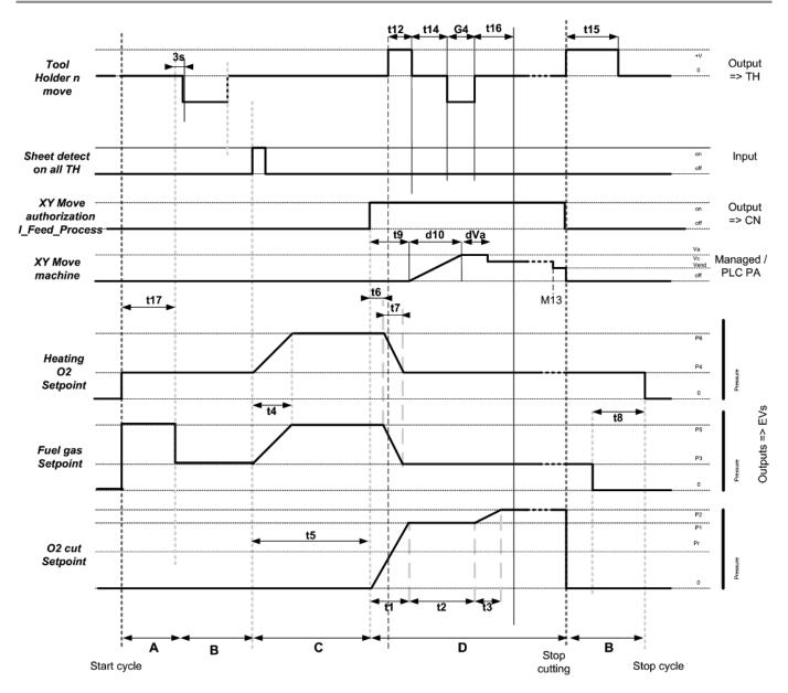
Above is a cycle for a machine with the ignition and sensing options activated
