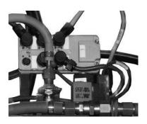
This assembly is present for each installed torch. It is assembled on the tool holder carriage.
