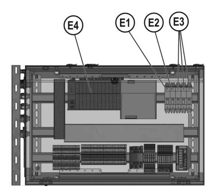
The fuses « E1 » (FU2) switch off the 230V supply to the 24VDC and 12VDC power supplies. (Description: FUSE 10X38 2A GG)
