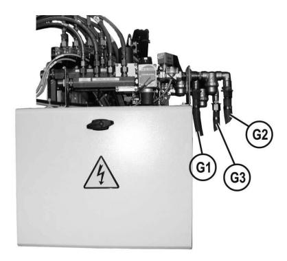
The pipes pass in the longitudinal chain, then behind the beam, for connection to the manifold.
