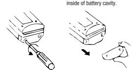
If the wire feed speed meter is not to be used for several months, remove batteries from the unit to prevent corrosion.
