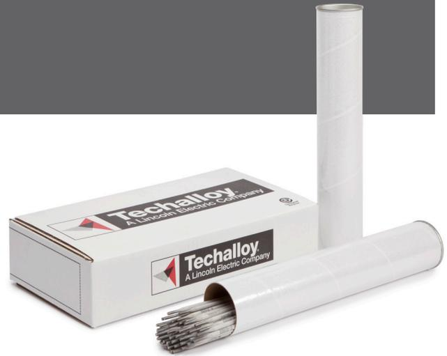
**Tech-Rod® 310** electrodes are used for welding stainless steels of similar composition in cast and wrought forms. The weld deposit is fully austenitic, and as such, calls for minimal heat input during welding.
