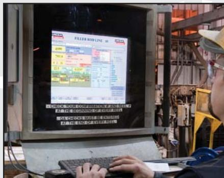
Moisture levels are monitored throughout processing, and lubricants are carefully selected to provide controlled diffusible hydrogen levels.
