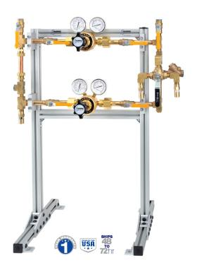
**The Model 1030** is a high flow gas supply manifold intended to be attached downstream of a bulk gas system/vaporizer and which will regulate the pressure and flow of gas into facility pipelines. The manifold utilizes the Harris Model 3550-250 regulators with stainless steel diaphragms. Flow rates up to 10,000 scfh can be achieved at the nominal inlet pressure of 350 psi. The system has a 450 psi maximum rated inlet pressure.
