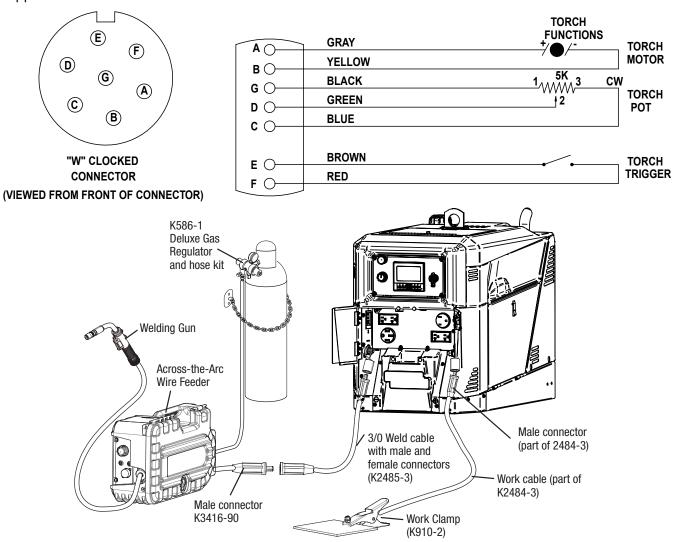
Figure 7: Across the Arc Feeder Setup - Electrode Negative (-) shown
