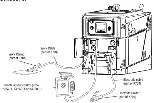
Figure 4: Standard Stick Setup - Electrode Positive (+) shown
