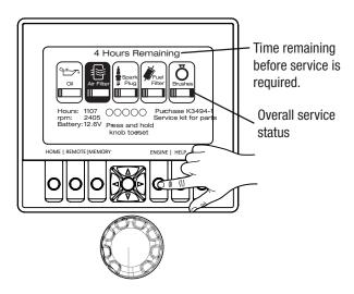
Five parts of the engine are monitored for service: Oil and oil filter, Air Filter, Spark Plug and Brushes. To view detailed information about an item, rotate the knob until the item is highlighted in red. The top of the screen displays the number of hours remaining until service is required for the selected item.
