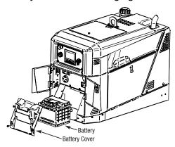
Figure 2: BATTERY CONNECTION
