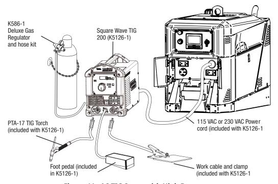
Figure 11: AC TIG Setup with High Frequency
