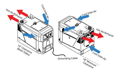
Figure 1: SERVICE TRUCK AND TRAILER INSTALLATION
