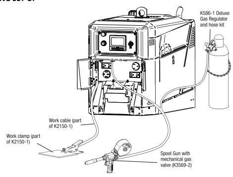
Figure 6: Spool Gun Setup - Electrode Positive (+) shown
