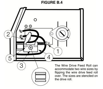
6. The idle roll pressure adjustment wing nut is normally set for mid-position on the pressure arm threads. If feeding problems occur because the wire is flattened excessively, turn the pressure adjustment counter-clockwise to reduce distortion of the wire. Slightly less pressure may be required when using 0.023 – 0.025" (0,6 mm) wire. If the drive roll slips while feeding wire, the pressure should be increased until the wire feeds properly.
