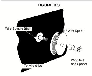
**Note:** The brake should be adjusted with a spool of wire installed. When properly adjusted it should move freely but not coast.
