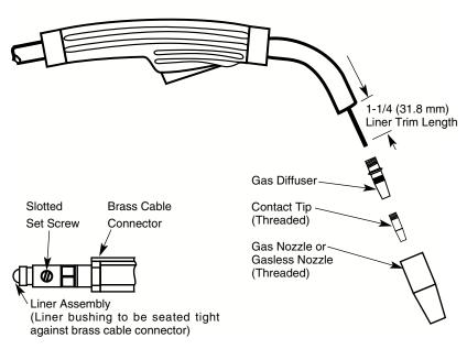
FIGURE D.2 Liner trim length for gun with <u>red trigger</u> (Magnum™ 100L)
