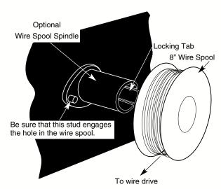
Wire Spool must be pushed all the way on the spindle so that the spindle's tab will hold it in place. The Wire Spool must rotate clockwise when wire is dereeled.
