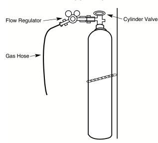
With the cylinder securely installed, remove the cylinder cap. Stand to one side away from the outlet and open the cylinder valve very slightly for an instant. This blows away any dust or dirt which may have accumulated in the valve outlet.
