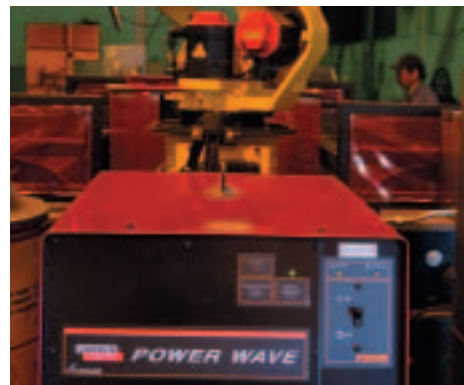
The Lincoln Power Wave® 455M uses ArcLink™, DeviceNet and Ethernet to communicate digitally with other welding system components, shop systems and via the internet for remote production monitoring.
