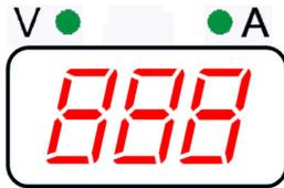
If the A LED is ON the meter displays the preset welding current (A) before welding and the actual welding current during welding. If the V LED is ON the meter shows the voltage (V) at the output leads. To switch between Current and Voltage visualization:
