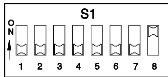
Figure F.50 - User interface board DIP switch location and position
