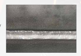
Moreover the stability given by this transfer allows to weld in all positions and especially in vertical up without weaving when it is associated to a MECHAPulse<sup>TM</sup> welding mode.
