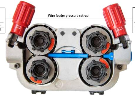
Steel 3-5 Stainless steel Braze 2.5-3.5 Flux cored 1.5-2.5 Aluminium
