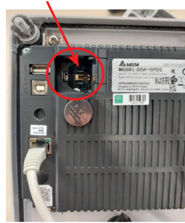
on the Delta HMI screen: CR2032 - 3V battery
