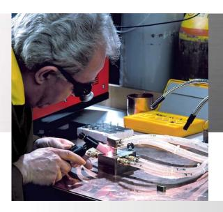
The micro plasma arc created by the combination of a current and a gas, concentrated by means of a nozzle, allows the use in welding of a high energy on a reduced surface.
