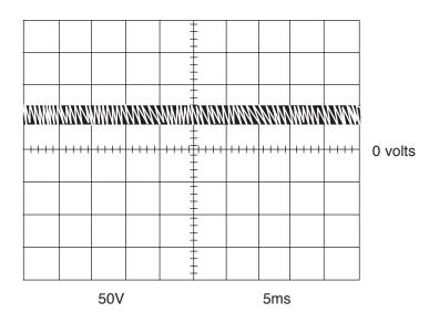
This is the typical DC open circuit output voltage generated from a properly operating machine. Note that each vertical division represents 50 volts and that each horizontal division represents 5 milliseconds in time.
