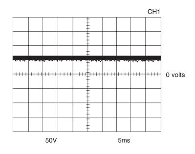
This is the typical DC open circuit output voltage generated from a properly operating machine. Note that each vertical division represents 50 volts and that each horizontal division represents 5 milliseconds in time.
