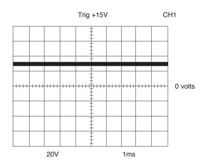
This is the typical DC output voltage generated from a properly operating machine. Note that each vertical division represents 20 volts and that each horizontal division represents 1 millisecond in time.
