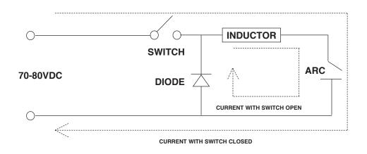
When the switch is closed, current is applied through the inductor to the arc. When the switch opens, current stored in the inductor sustains flow in the arc and through the diode. The repetition rate of switch closure is 20Khz, which allows ultra-fast control of the
