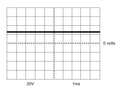
This is the typical DC voltage generated from a properly operating machine. Note that each vertical division represents 20 volts and that each horizontal division represents 1 millisecond in time.
