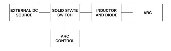
In this system, the engine drives a three-phase alternator, which generates power that is rectified and filtered to produce about 75VDC. The current is applied through a solid state switch to an inductor.
