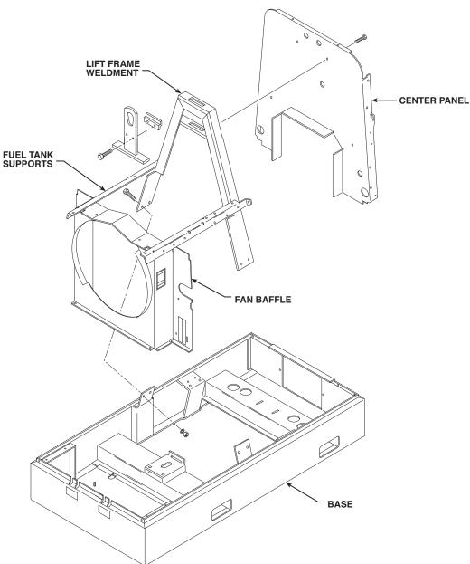
In steps 21 - 25, the lift frame weldment, fuel tank supports, and fan baffle are removed as a unit. See Figure F.23.
