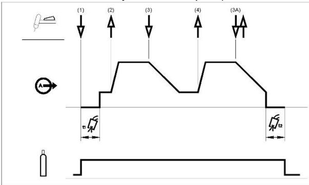
3. Press and hold the TIG torch trigger. The machine will now decrease the output current at a controlled rate, or downslope time, until the Crater current is reached.
