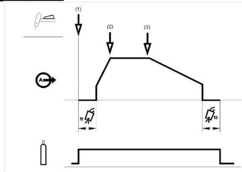
In Spot sequence, the trigger (step 1) starts the welding sequence. Unlike other parameters, the end of cycle does not depend of trigger action: a time set on UI will initiate automatically the slope down phase.
