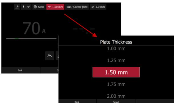
Once parameters are modified, the output welding current will be automatically adjust to fit with the application.
