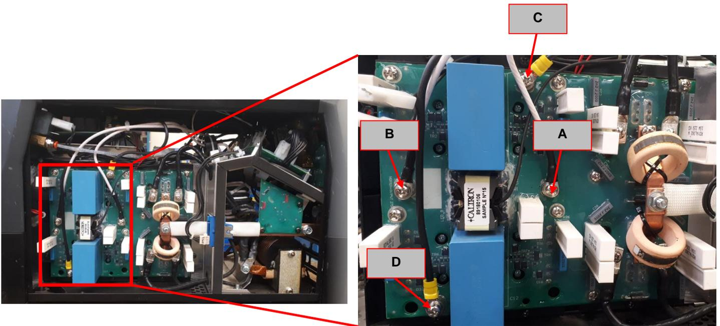
**Figure 4 – Inverter Board location and Test Points**
