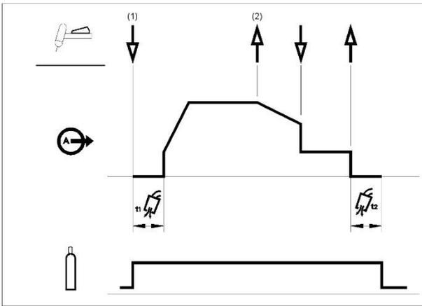
As shown above, it is possible to press and hold the TIG torch trigger a second time during downslope to end the downslope function and maintain the output current at the Crater current. When the TIG torch trigger is released the output will turn OFF and the post flow time will start. This operation sequence, 2-step with restart disabled, is the default setting from the factory.
