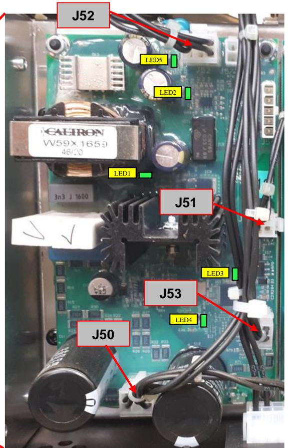
**Figure 12 – AUX. Power Supply Board location and Test**
