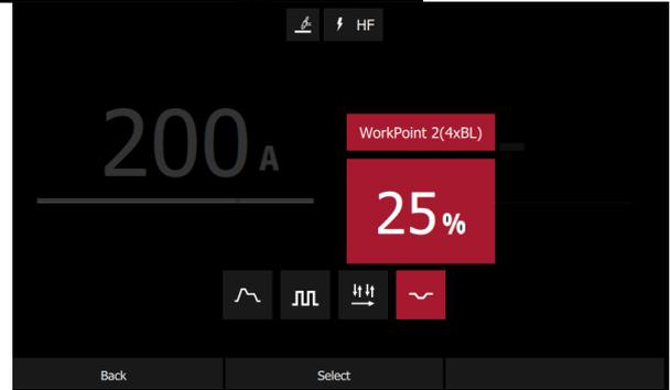
When this sequence is selected, a new icon appears on the right allowing to configure the second level current value. In this example, the background current level will be 25% of welding current value.
