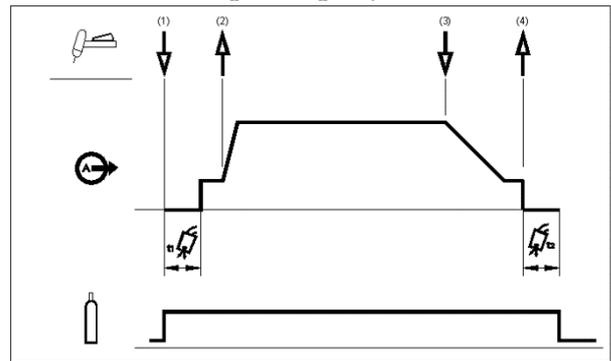
1. Press and hold the TIG torch trigger to start the sequence. The machine will open the gas valve to start the flow of the shielding gas. After the pre-flow time, to purge air from the torch hose, the output of the machine is turned ON. At this time the arc is started according to the selected welding mode. After the arc is started the output current will be at the Start current. This condition can be maintained as long as necessary.
