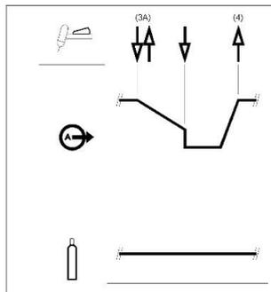
As shown here, again after the TIG torch trigger is quickly pressed and released from step 3A, it is possible to quickly press and release the TIG torch trigger a second time to end the downslope time and stop welding.
