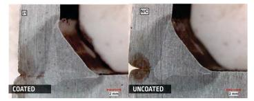
Micro-Etch testing shows no discernable weldment differences between uncoated  $\boldsymbol{\Theta}$  RP6 coated base material
