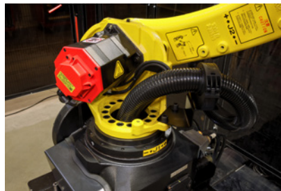
Enclosed cable connection
