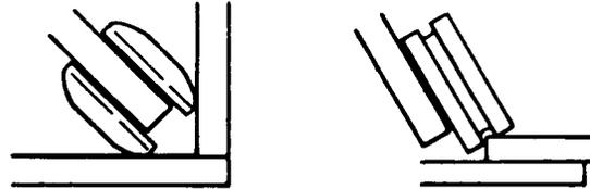
2. If making fillet welds, install the double guide rolls which are designed to ride against both the vertical and horizontal members of the joint with sufficient clearance between the rolls to clear tack welds.
