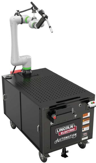
Cooper CRX-10iA/L Air-Cooled Wire-Brake Welding Cobot Cart
