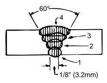
Successive passes must be used to build up butt welds on heavier metal.
