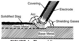
FIGURE 4. -The welding arc.
