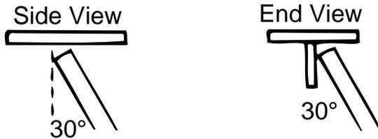
It is important to hold a VERY SHORT arc. (A long arc will result in falling molten metal; a short arc will make the metal stay.)
