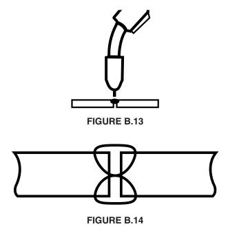
In the example shown in Figure B.14, the joint has been welded so that 100% penetration could be achieved. The weld, if properly made, is as strong as or stronger than the original metal.
