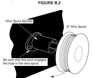
Wire Spool must be pushed all the way on the spindle so that the spindle's tab will hold it in place. The Wire Spool will rotate clockwise when wire is dereeled.
