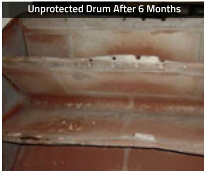
Vane pockets are damaged by wear and corrosion and must be replaced.
