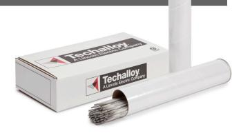
**Tech-Rod**® **308/308L** electrodes give a weld deposit, with reduced carbon levels (0.04% max) that offers increased resistance to inter-granular corrosion. Type 308L is ideal for welding Type 304L stainless steels.
