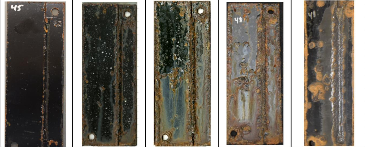
CV45 CV46 CV47 CV48 CV48 CCT 25 Cycles CCT 60 Cycles CCT 90 Cycles CCT 120 Cycles CCT 120 Cycles Rust Removed
