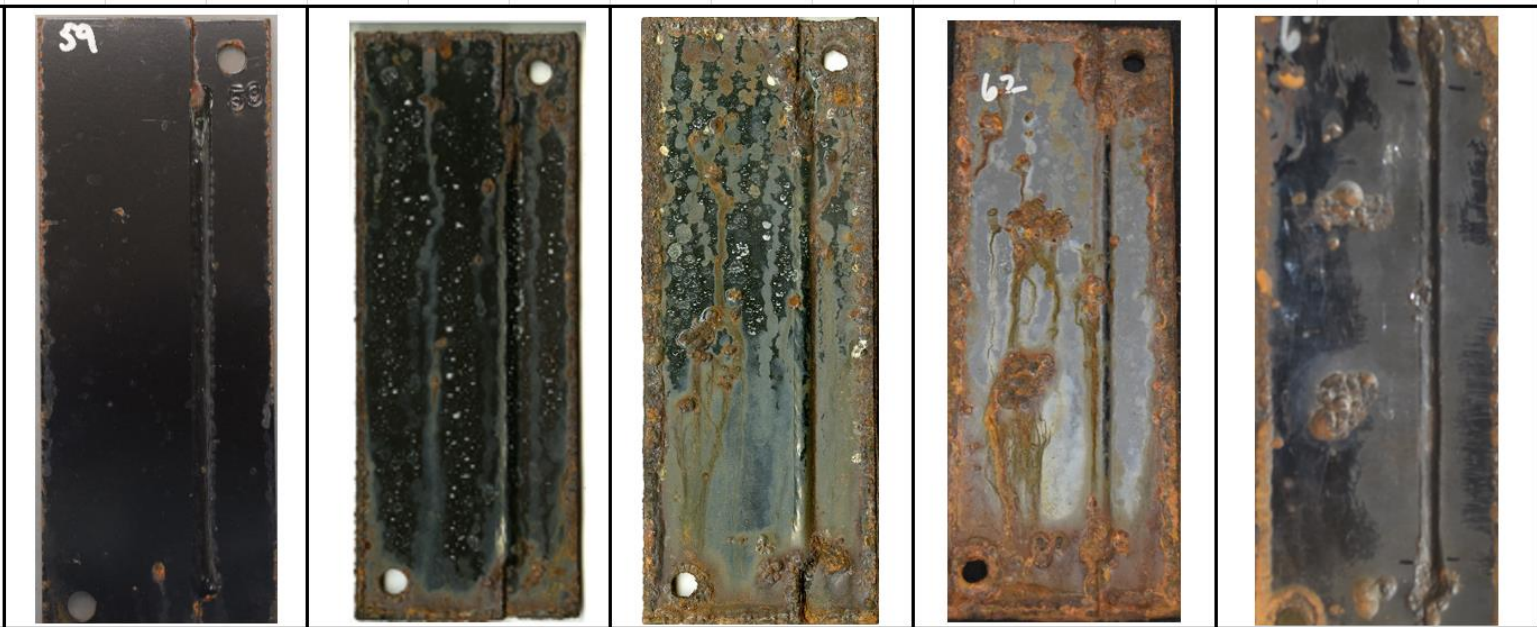
AV59 AV60 AV61 AV62 AV62 CCT 25 Cycles CCT 60 Cycles CCT 90 Cycles CCT 120 Cycles CCT 120 Cycles Rust Removed
