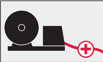
A positive (+) sense lead is required. This is a standard connection in an ArcLink® cable.
