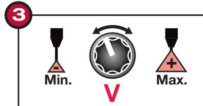
Adjusting voltage increases or decreases the arc length, allowing the user to fine tune arc characteristics.
