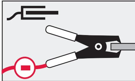
A negative sense lead (optional) is highly recommended for total welding cable lengths >50 ft. and should be connected directly to the workpiece.
