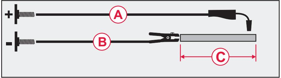
The total length of the welding current loop (A+B+C) should be minimized to reduce inductance.
