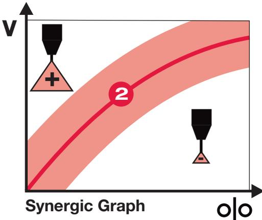
**Precision Pulse™** waveforms are synergic weld modes. Based on the wire feed speed ①, set by the operator, a pre-programmed voltage is automatically selected ②. Fine tune the arc length using Voltage.
