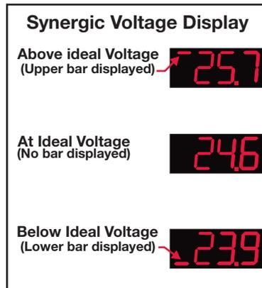
Synergic Weld modes improve the ease of set-up by pre-selecting an ideal voltage based on the selected WFS. The user can then fine tune their Voltage setting based on their personal preference and can easily see whether they are above or below the nominal setting.
