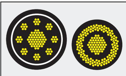
For configurations with excessive inductance, use Lincoln Electric® patented coaxial welding cables.
