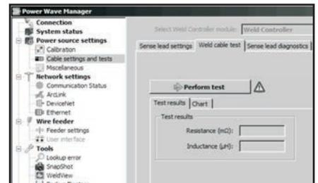
Test cable inductance levels using the Power Wave® Manager software exclusively from Lincoln Electric® Software is available at [www.powerwavesoftware.com](http://www.powerwavesoftware.com).
