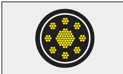
Lincoln Electric® coaxial cables combine the positive and negative welding leads into one cable to minimize cable inductance.
