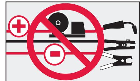
**DO NOT** route sense lead cable close to high current welding cables as this may distort the sense lead signal.
