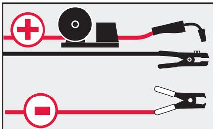
The negative sense lead should be separated away from welding cables to minimize interference.
