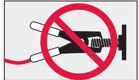
**DO NOT** connect either sense lead to a welding stud on the power source as this may result in erratic arc behavior.
