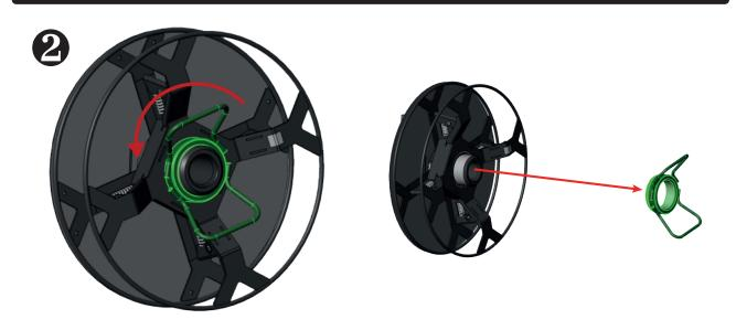
Unscrew and remove the locking nut 95093534
