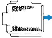
If your air cleaner has a safety filter, replace it every third primary filter change. Remove the safety filter as you would the primary filter. Make sure you cover the air cleaner outlet tube to avoid any unfiltered contaminant dropping into the engine.
