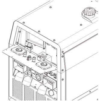
Locate VRD switches (as marked in Fig A.2) on both PC control boards. Left position on each switch indicates "OFF" state; right position on each switch indicates "ON" state. PC Control Board on the left is for settings for the left user. PC Control board on the right is for settings for the right user.
