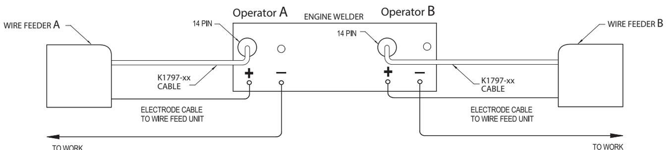
**CONNECTION OF ACROSS THE ARC WIRE FEEDERS TO THE DUAL MAVERICK® 200/200X**
