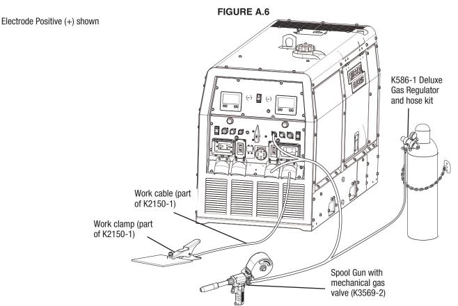
In the spool gun mode, the weld output is controlled by the trigger of the spool gun. The knob on the Dual Maverick display sets voltage and the spool gun knob sets wire feed speed. Rotating the knob on the spool gun adjusts the work point (wire feed speed). Spool gun modes have the option of being "synergic" (when the wire feed speed is changed, the voltage is automatically modified up or down to maintain a similar arc length).
