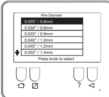
NOTE: After selecting Synergic Control, the user is required to select their desired Wire Type and Wire Diameter. This allows the program to calculate the recommended range for their welding needs.
