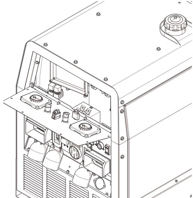
4. Locate VRD switches (as marked in Fig A.2) on both PC control boards. Left position on each switch indicates "OFF" state; right position on each switch indicates "ON" state. PC Control Board on the left is for settings for the left user. PC Control board on the right is for settings for the right user.
