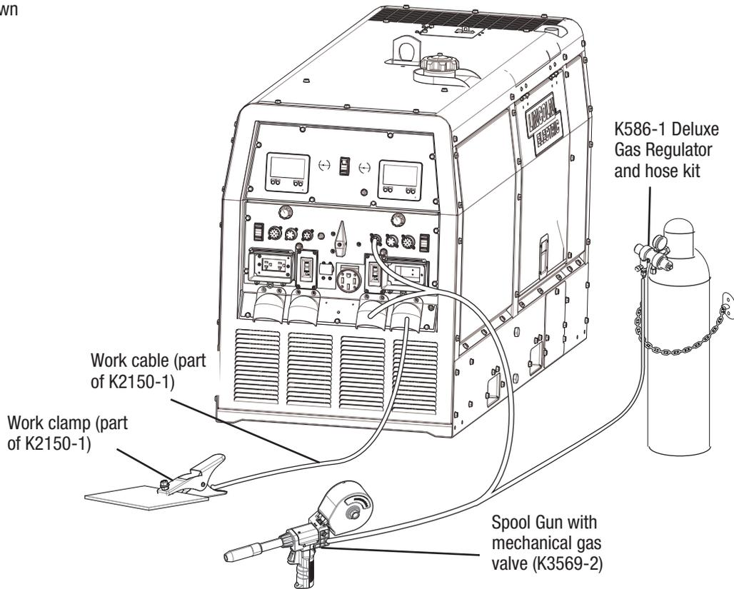
In the spool gun mode, the weld output is controlled by the trigger of the spool gun. The knob on the Dual Maverick display sets voltage and the spool gun knob sets wire feed speed. Rotating the knob on the spool gun adjusts the work point (wire feed speed). Spool gun modes have the option of being “synergic” (when the wire feed speed is changed, the voltage is automatically modified up or down to maintain a similar arc length).
