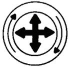
Rotate the filter while pulling straight out.
