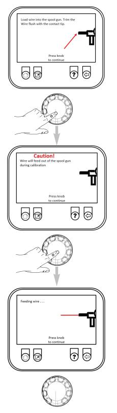
This screen will remain for approximately 5 seconds as the wire feeds. During this process, the wire coming out of the spool gun will grow longer as a visual representative.
