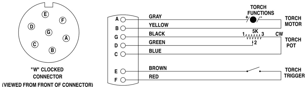
**CONNECTION OF WIRE FEEDERS WITH CONTROL CABLE (14 PIN)**
