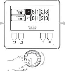
Rotate the knob to adjust the value of the PIN. Press the knob to advance to the next number. Press the BACK button to go the previous number.
