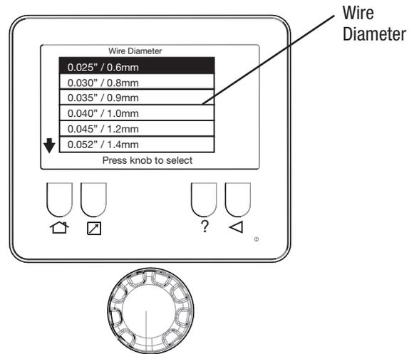
**Note:** Select the maximum wire feed speed (WFS) that will be used during the welding session to ensure power output to the wire feeder is sufficient.
