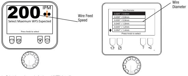
Note: Select the maximum wire feed speed (WFS) that will be used during the welding session to ensure power output to the wire feeder is sufficient.
