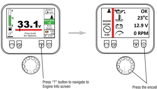
Press the encoder knob or the back button to return to previous screen
