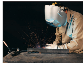
STT® using CO 2 and .045" solid wire. Note reduced spatter and fume.
