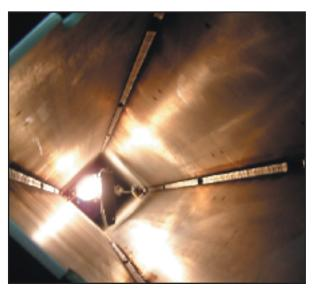
The design also called for tight final dimensional tolerances, since the basket assembly sits inside of a canister that ultimately slides into an exterior cask. These measures safeguard against leakage of radioactive material but also dictate that shrinkage and distortion resulting from the welding process be kept to a minimum.
