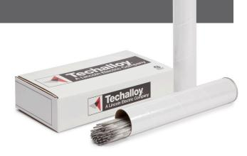
**Tech-Rod**® **312** is used to weld cast and wrought alloys of similar compositions. The electrode can also be used for joining hard to weld materials and dissimilar metals. Applications should be limited to 800°F (420°C). The weld deposits exhibit high tensile strength and offer some resistance to abrasion.
